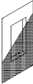
Step 1: Apply continuous weather barrier over window opening.
